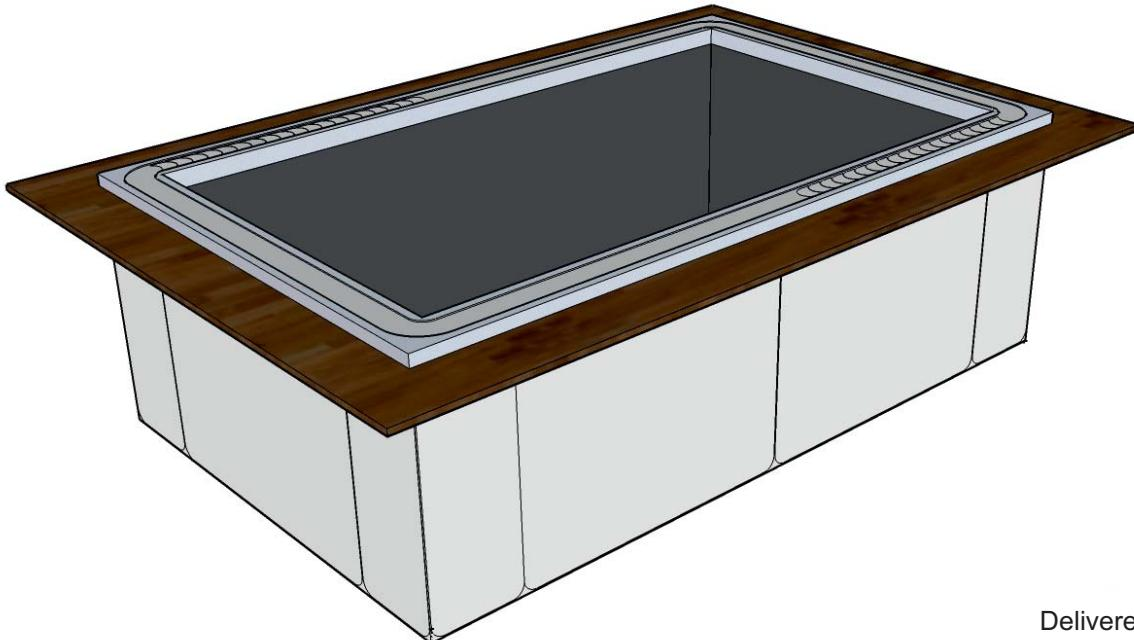
Layout E1. 2500mm x 2500mm single lane, 1050mm to the floor.
